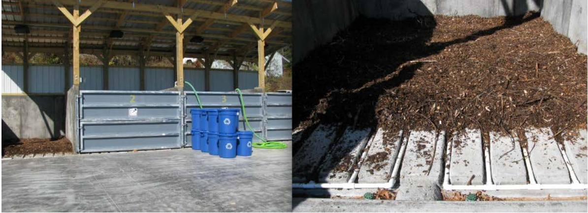
Figure 7. Covered aerated bin composting at Appalachian State University.
