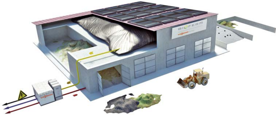
Figure 10. Schematic of dry fermentation system of BioFerm (Mckiernan, 2012, p. 4).
